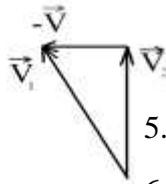
5.  $v_1 = \sqrt{v_2^2 + v^2}$
